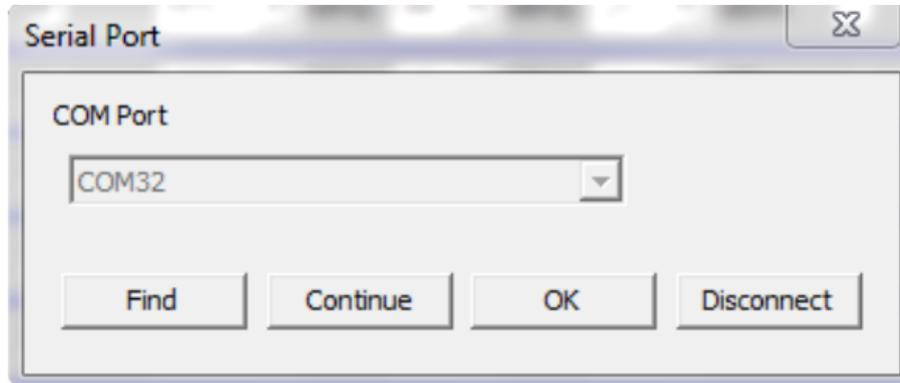
„**Find**” – It starts searching for serial port and connected dController to it.
