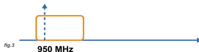
**“UB freq. exceeds L-Band range”** – The user band center frequency has been set out of range of 950 and 2150 MHz.
