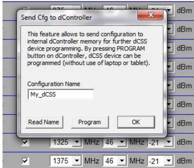
**„Configuration Name”** – A field to give a name to the UB settings from main window.
