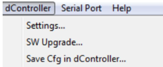
**“Settings...”** – It opens a menu for dController settings (SW version, output voltage).
