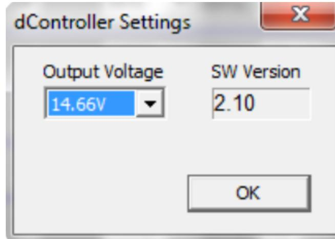
„**Output voltage**” – It displays current voltage and allows to set new voltage on output.
