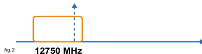
**“UB bandwidth out of range”** - The user band bandwidth has been set out of range of 24 and 82 MHz.
